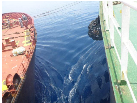
Improper placement of Secondary Fender
