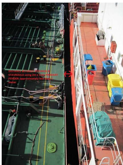
*Fenders of small diameter will reduce ship distance and increase the risk of collision and mooring lines breakdown*
